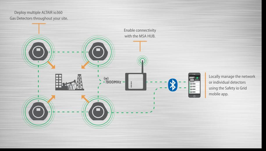
Each MSA HUB can support up to 32 ALTAIR io360 Gas Detectors. The 868 MHz HUB (Europe and Middle East) supports up to 16 detectors.
